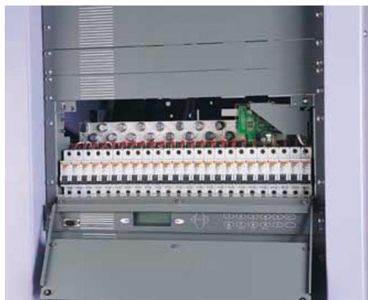
The Intergy DCM range of Miniature Circuit Breaker (MCBs) DC distributions provides circuit protection for a wide selection of telecommunications loads up to 1200A. All MCBS are alarmed with automatic detection of load current to prevent false alarms from unused MCBS.
